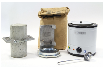
Cylinder capping equipment: cylinder carrier 55-C0121/3, vertical cylinder capper 55-C0121/21, capping compound 55-C0121/37, stainless steel ladle 55-C0121/5 and Melting pot, 5 liters cap. 55-
