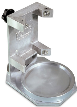
Vertical cylinder capper for 160x320 mm specimens complete with ball tracks for a positive location of the specimen, model 55-C0121/22A
